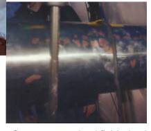
Copper areas are hand finished and then flashed with nickel tungsten to acquire hardness.
